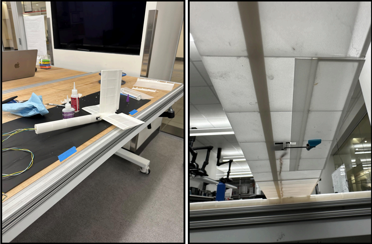
Figure 13/14. Aircraft empennage, wing servo and control surface
